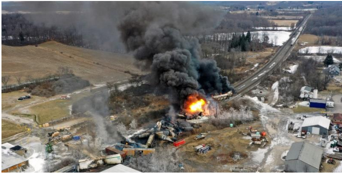
Figure 2: Aerial view of the East Palestine, Ohio train derailment, involving 149 train cars—38 of which derailed—with 11 tank cars igniting containing hazardous materials.
