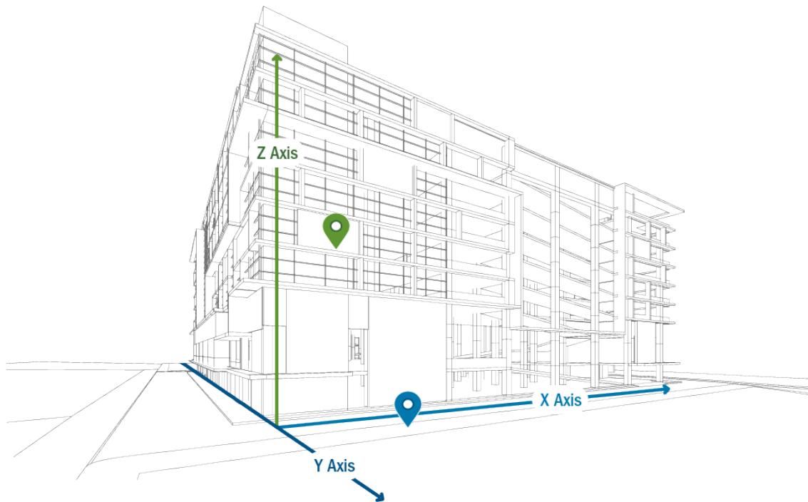
Figure 4: Example of Z-Axis Coordinate Providing Vertical Location of Subscriber Unit
