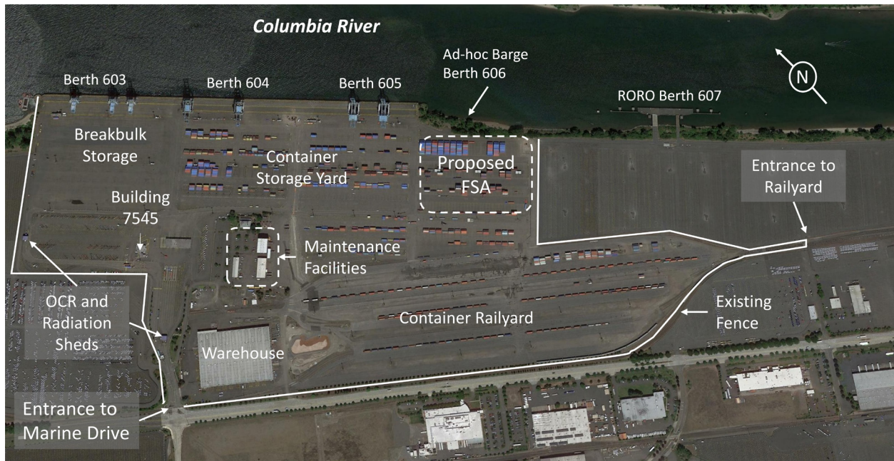
Figure 1: Terminal 6 Container Yard Layout.
